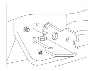
12. Fit the cross tube between the side arms. Insert a spacer between each side arm and the cross tube.
