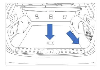
20. Remove the RHS foam insert by removing 2x scrivets.
