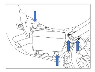
8. Remove 4x screws from the heat shield to access the chassis mount hole.
