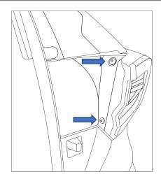
Remove 2x screws. Pull the taillight rear ward and disconnect the wire.
