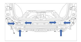
11. Insert the side arm into the chassis and loosely secure with 3x M14 bolt and 3x washer.
