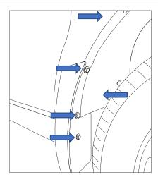
Remove 2x scrivet clips on bottom edge. Remove mudflap assembly. Remove final scrivet from bumper edge after removal of mudflap.
