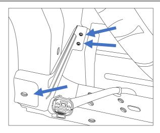
3. Attach sidearm to chassis rail using 6 x M14 bolts (2 x 45mm in vertical direction & 4 x 35mm in horizontal direction) complete with 1 x washer per bolt.
