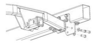
6. Secure bumper to bumper tabs using 1 x M6 bolt per tab, complete with 1 x nut and 2 x washers per bolt.
