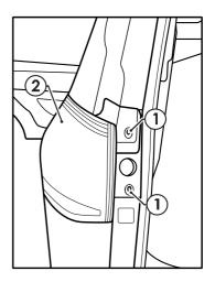
23. At the LHS tail light, unseat the tail light harness grommet (1) and push through the hole and into the vehicle.
