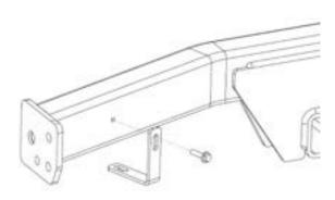
5. Using two people, raise centre section up to sidearms. Attach with 3 x M12 bolts per side, complete with nuts and washers.
