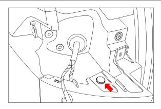
4. In wheel arch remove 4 x screws and 1 x plastic screw from the underside of bumper.
