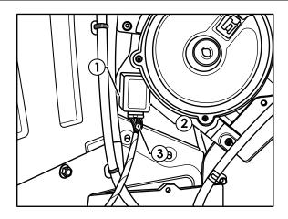
27. Drill a 30mm grommet hole (1) in a suitable location to enable the tail harness to be routed from the towbar to the ECU.
