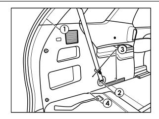
15. Position the towbar onto vehicle with the sidearms going into the chassis rail. Loosely secure each side to the back panel captive nuts with 2 x M10 bolts complete with 1 x washer per bolt.
