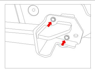
16. Position the support plate under the chassis rail and loosely secure with 2 x M12 bolts complete with 1 x washer per bolt and to the back panel with 1 x M12 bolt complete with 2 x washers and 1 x nut per bolt.
