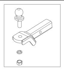
2 .Fit TBM assembly to the towbar hitch receiver in the upward-position and secure with PullPin. Ensure to fit the R-Clip to the Pull Pin.
