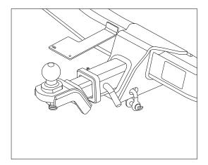
3. Affix the TBM kit compliance label onto the towbar.
