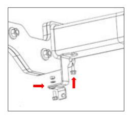
18. Secure the bracket to the towbar using a screw. Secure the antenna to the bracket using 2x screws and 2x nuts.
