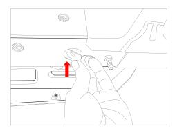
11. Fit the LHS side arm and loosely secure with 3x M12 bolts and 3x M12 washers.
