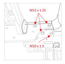
12. Fit the LHS side arm and loosely secure with 3x M12 bolts and 3x M12 washers.
