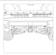
15. Remove the wire harness by cutting the wire fir tree clips on the impact beam. Unclip 5x scrivets from the impact beam. Remove 2x screws and disconnect the antenna.
