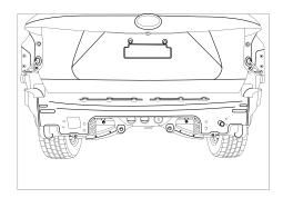
9. Remove the exhaust muffler by unscrew 2x bolts and slide off 3x rubber muffler hangers.
