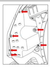
6. On the RHS below the wheel arch. Remove 3x scrivet clips.
