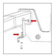
17. On RHS, secure the bumper tab bracket to the towbar using a Tek screw.
