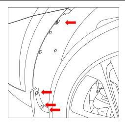
5. On the LHS below the wheel arch. Remove 4x scrivet clips and 2x plastic nuts.
