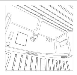
2. Remove 2x screws and pull the taillight rearward.
