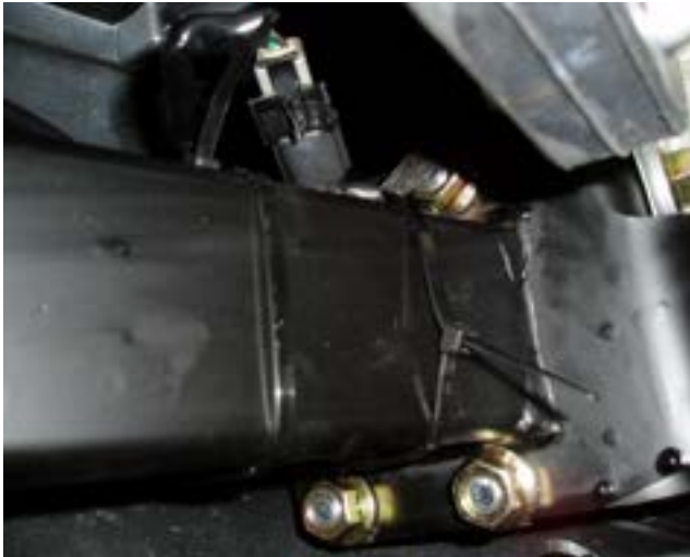
Fig 5: Shows the heat shields to be trimmed.
