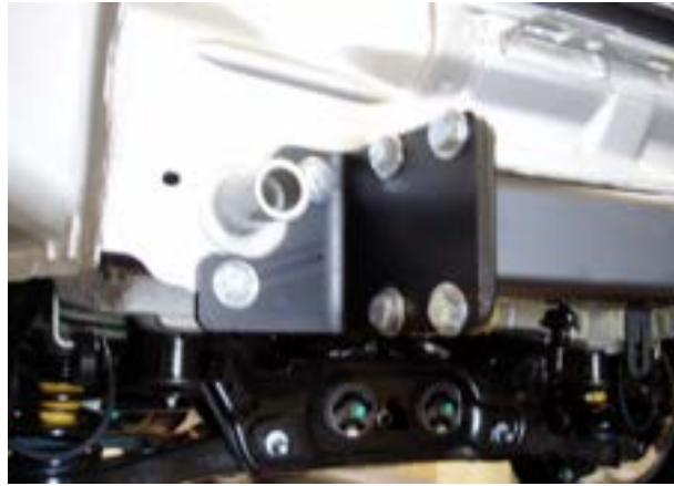
Fig 4: Shows lower bumper being attached.
