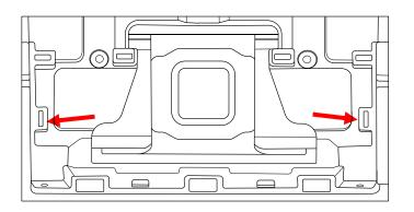
3. Fit TBM inside cavity on the back of the vehicle.
