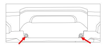
2. Push the two catches outboard to release the cover.
