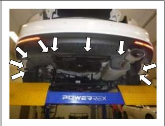
**9.** Under vehicle on LH side, remove 4x nuts and remove the tyre well protector.
