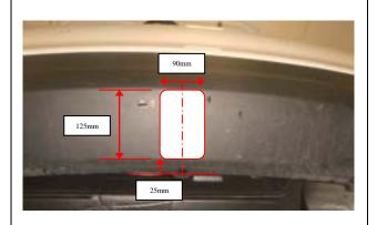
**16.** At an appropriate position on the bumper, mark out and drill 2x ø5mm holes 69mm apart on bumper skin to support plug bracket.
