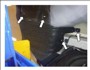
**10.** From underneath vehicle, remove 4x bolts (2 per side) securing bumper assembly (impact beam) to vehicle rear panel.
