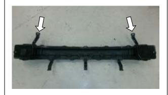
**12.** Mount towbar assembly to vehicle, secure with 4 x M10 bolts complete with washer.
