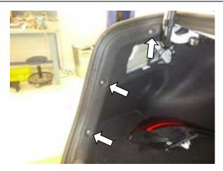
**6.** On the LH side, peel away boot lining to expose the harness connector. Reach in and disconnect the plug.
