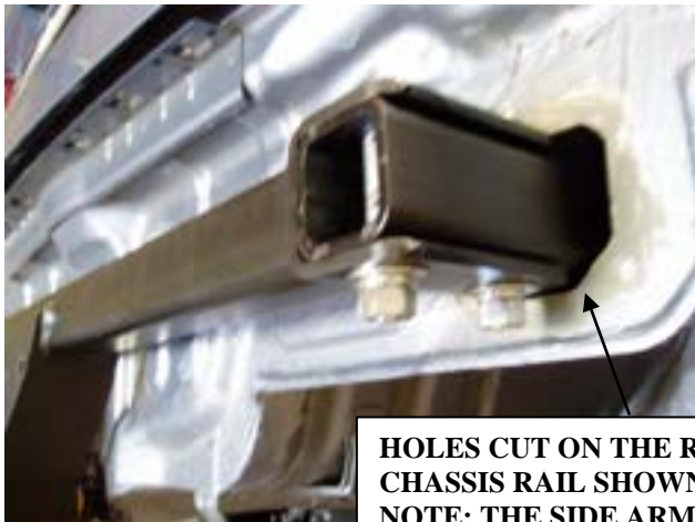
Fig 1: Shows holes cut on rear panel, side arms inserted & towbar bolted on.
