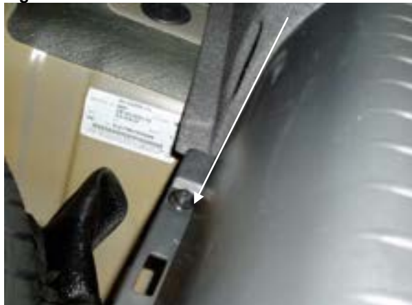
Fig 8: Remove 4 bolts as shown from inside of boot.
