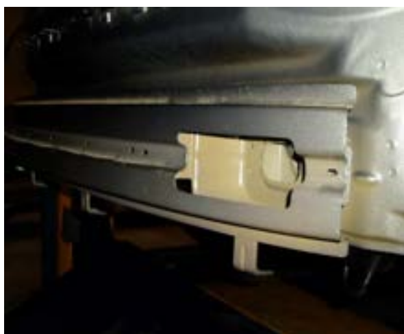
Fig 10: Remove & discard impact beam shown.
