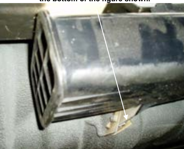
Fig 11: Remove charcoal canister, by removing bolt at the bottom of the figure shown.
