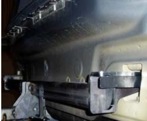
Fig 15: shows towbar mounted from inside of boot.
