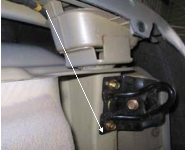
Fig 14: Line up the packer assembly as shown below.
