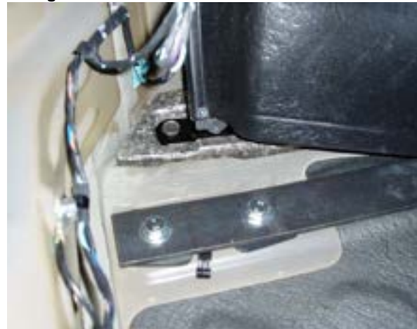
Fig 16: Shows towbar being mounted up from bottom of chassis.
