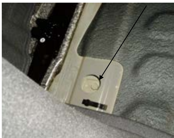
Fig 10: Remove & discard impact beam shown.
