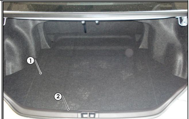
2. Remove the LHS and RHS tool storage compartment (1) and the centre wheel cover (2).
