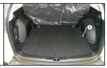
2. Remove the two plastic clips (1) and then remove the rear luggage compartment trim (2) by pulling in an upwards direction.
