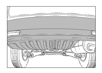
8. Remove the Bumper Cover via 3x Bolts as shown in the picture and Store them in a safe Location after removal.
