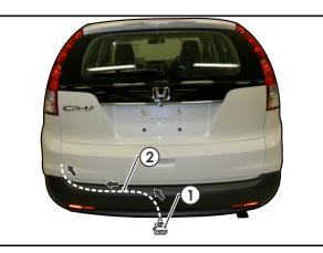
**19.** Connect the tail harness (tail length 1800mm) 8-way connector (1) to the trailer patch mating 8-way connector (2).
