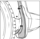
2. Remove 1 x Clip and 3x Screws to remove the Driver Side Rear Mud Guard as shown.
