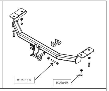
11. Torque all fasteners to specification on Page 2.
