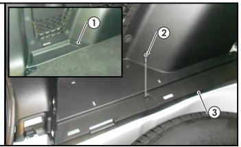
**10.** On the LHS rear quarter of the vehicle, drill out the existing grommet (1) to Ø30mm.
