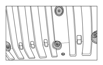
9. Lower the Exhaust to gain better access as shown by removing the two Muffler Bushings from the Vehicle Pins.
