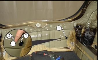
**16.** Route the trailer patch (P/No: 100822-WL) **(1)** up along the LHS vehicle harness towards the tail light connectors.
