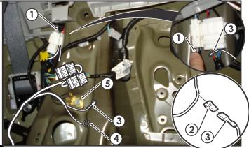
**20.** Route the trailer patch (P/No: 100822-WL) **(1)** along the rear of the luggage compartment area towards the RHS tail light connector area.
