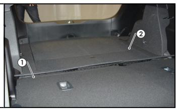
3. Remove the spare wheel (1) by removing the spare wheel fastener (2).
