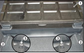
8. Remove the centre divider (1) by removing the two fasteners (2).
