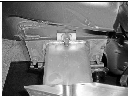
Figure 4 – Remove Impact beam from back panel.
