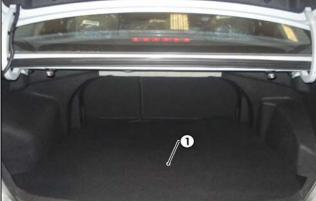
2. Remove the rear trim (1) by first removing the two fasteners (2).
