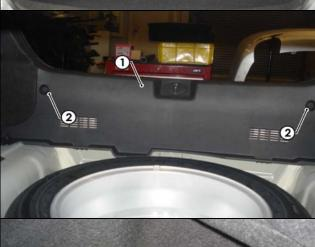
3. On the RHS of the luggage compartment, remove the rear storage tray (1) by first removing the fasteners.
