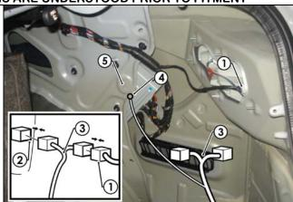
28.In the luggage compartment, connect the tail harness connector (1) to the trailer patch harness mating connector (2).
