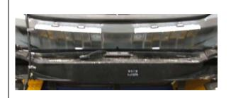
Remove impact beam and discard, remove sensor to be reattach to towbar.
