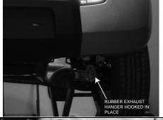
5. Disconnect rear muffler hangers to lower the muffler.
