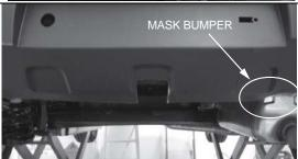
7. Remove the centre bumper hanger and discard. From centre of bumper cut 90mm wide 175mm long for towbar cutout.
