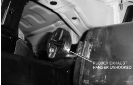
6. Disconnect front muffler hangers to lower the muffler
