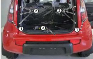
2. Connect the Trailer Patch Harness (P/No: 100149-WL) (1) to the vehicle tail light connectors (2).
