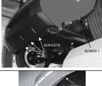
2. Remove 3 scrivets from the underside of the vehicle.
