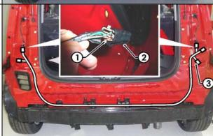
On the Tail Harness and mating connector, apply electrical grease or silicon (1) on to the back of the connectors to make them water proof.
