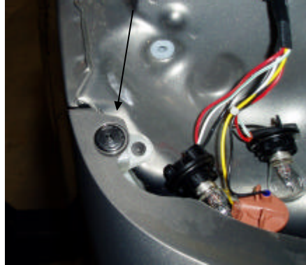
Fig 7: Remove rubber plugs shown below.
