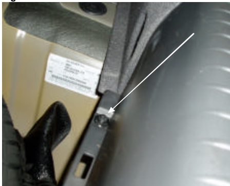
Fig 8: Remove 4 bolts as shown from inside of boot. using
