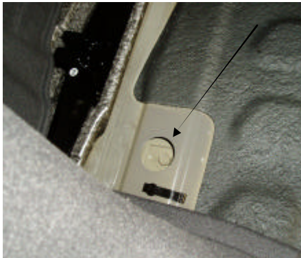
Fig 8: Remove 4 bolts as shown from inside of boot. using
