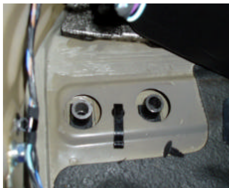
Fig 16: Shows towbar being mounted up from bottom bumper of chassis.
