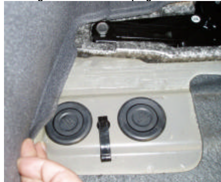
Fig 9: Remove wiring & wrap it around towbar cable ties provided if necessary.
