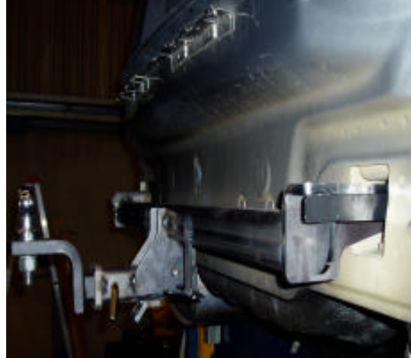
Fig 15: shows towbar mounted from inside of boot.
