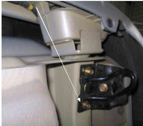
Fig 14: Line up the packer assembly as shown below. boot.
