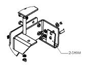
CHASSIS BRACKET ASSEMBLY FOR 2004 ON MODELS FIT SHIM AS REQUIRED
