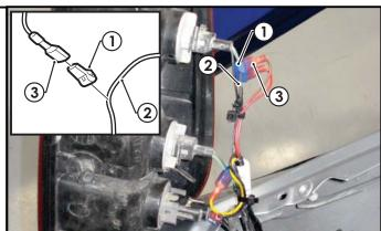
3. Connect the Trailer Harness ground ring terminal (1) to the LHS vehicle grounding point (2).
